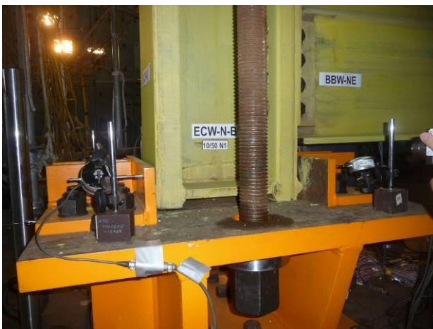
Figure 7: Pseudo-dynamic test: (a) Global view showing scale of specimen; (b) Parts of test set-up; (c) Rocking pre-tensioned column case, and; (d) Anchorage point of column pre-tension
